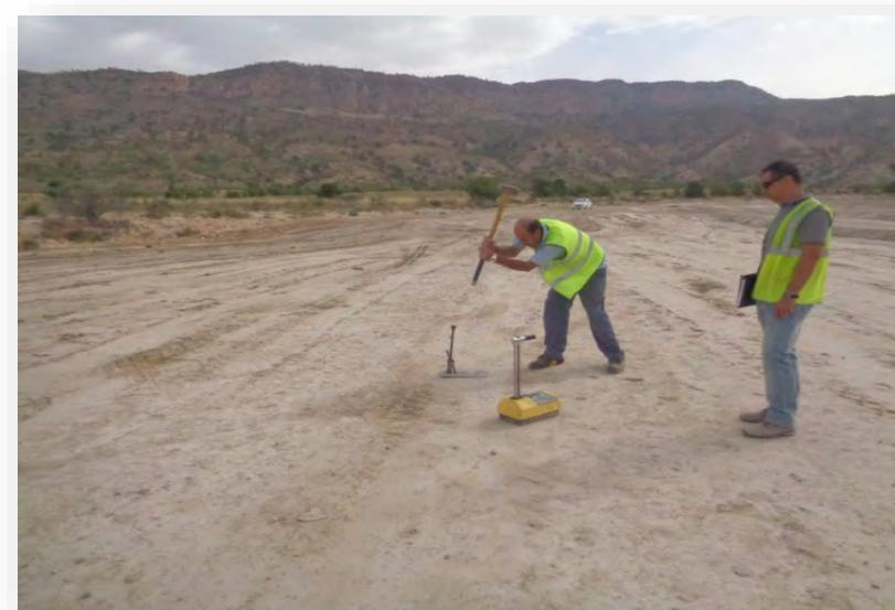
DENSIDAD "IN SITU" MEDIANTE SONDA NUCLEAR.
